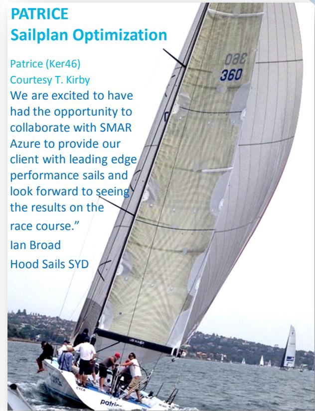
The goal was to optimize the sail plan for a new Ker46 that was in production. Using the SMAR Azure sail design and performance analysis tools, the SMAR Azure team optimised sail shapes and the fiber layouts in the given range of wind conditions.
